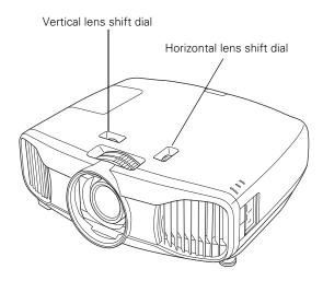
**Caution:** Do not try to move the lens by hand, or you may damage the projector. Always use the lens shift dials to change the lens position.
